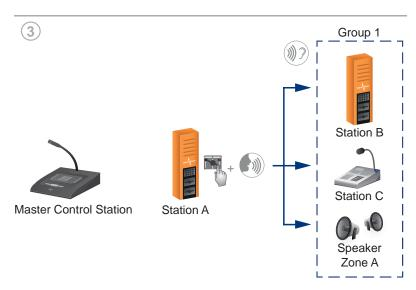
A temporary PA connection is configured. Subscriber at Station A presses the switchboard speak key, keeps it pressed and makes an announcement.
